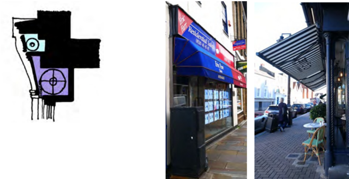
Figure 26 (left) - Section through a traditional fascia with integral roller blind (blue) and roller security shutters (purple). Figure 27 (right) - Dutch v simple roller blinds.
